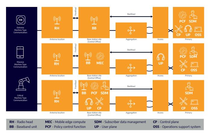
Figure 2: Service component VNF locations in relation to the user for different service types.
